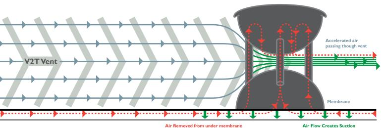
The V2T Roof System is steadily becoming the standard roofing system for low-slope roofs across the United States. This is because V2T installs faster, more easily, uses less materials, is more environmentally friendly and still carries 20-year warranties from major roof membrane manufacturers such as Carlisle, Fiber-Tite, Flex, Versico and others.
